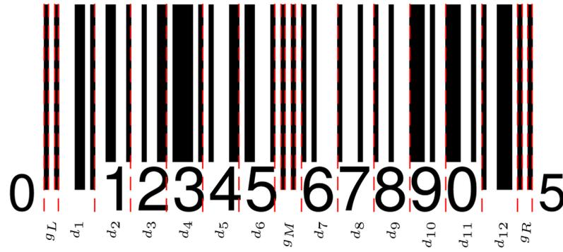
**Figure 2.** Fixed edges of UPC-A barcode shown as dashed red lines. Labels on bottom denote the guard regions and the 12 digit regions between the fixed edges.
