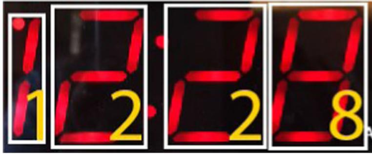
**Figure 1.** Sample LED display contains a string of digits, each of which is a standard seven-segment digit. For each digit, our algorithm estimates its bounding box (shown in white) and then reads it (results in yellow).
